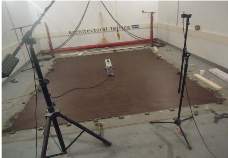
Source Room View of Test Specimen Installation
